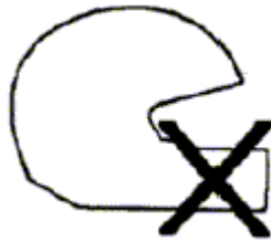
Figure 1: Approved symbol for lower face cover that does not protect chin from impacts
